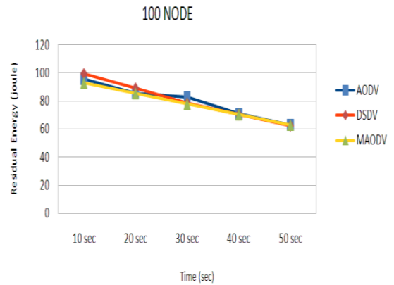
Figure:- Residual Energy for 100 nodes under AODV, DSDV and MAODV
