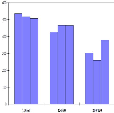
Figure 4: Influence of specimen geometry (lower span/upper span) on initiation values of GIIC (in J/m<sup>2</sup>) from mode I precrack, brittle carbon/epoxy specimens 3 mm thick, results from K. Tanaka, University of Toyama, 2nd VAMAS Mode II round robin tests.
