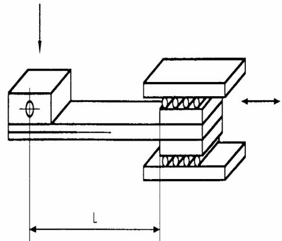
Figure 6: Schematic of the End Loaded Split test set-up for mode II delimitation resistance testing.
