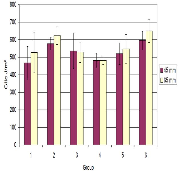
Figure 5: Propagation values measured by 6 groups at two crack lengths for carbon/epoxy,
