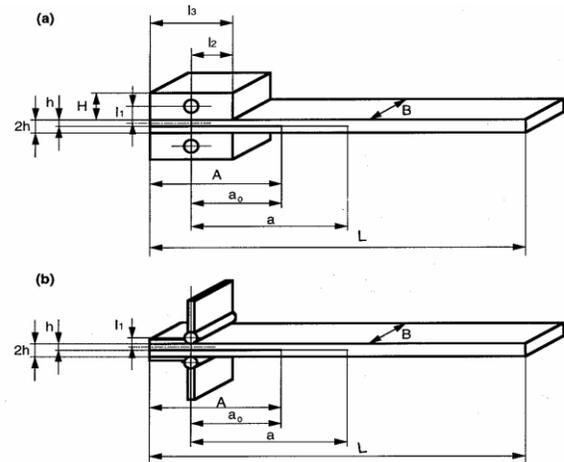
Figure 1: Schematic of the Double Cantilever Beam specimen used for Mode I testing, load blocks (a) or piano hinges (b) can be used for the load introduction [6].
