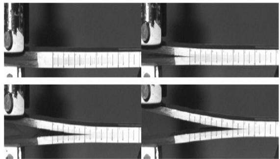
Figure 3: A series of frames selected from a high speed video sequence recorded at 4000 frames per second. The time interval between each frame shown here is 5 ms (in the film sequence, the frame interval was  $250\mu\text{s}$ ). The photographs are from a DCB-test at 1 m/s and even at this relatively moderate loading-rate, an asymmetry is introduced.
