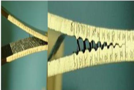
Figure 2: Typical delimitation path observed in cross-ply (alternating  $0^\circ/90^\circ$  layers) laminates, oscillating between adjacent  $0^\circ$  plies. (Left): view onto fracture surface. (Right): edge view. If delimitation paths deviate into the  $0^\circ$  plies tests are considered invalid.
