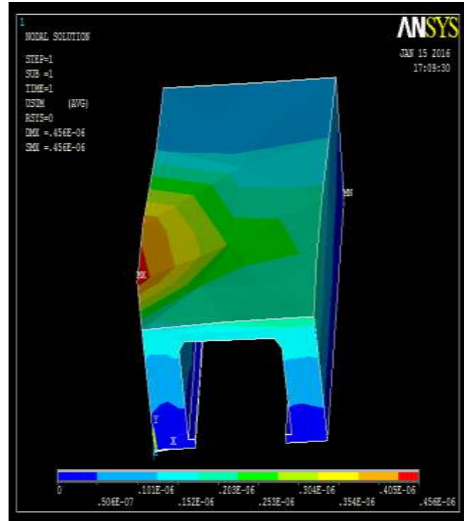
Figure 7 Displacement of bridge when load at node 209
