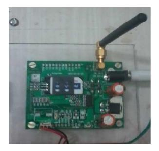
The system is shown in figure below. It is main station board which has two connecters, first is connected to GSM module and other is connected to PC through serial cable. The GSM module receives data from node; send it to PC through microcontroller.
