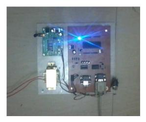
It is data monitoring node which is connected to sensors, and a GSM module using serial cable. An LCD is also connected with this board to display the data which it receives from sensors.
