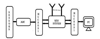
The Measuring Parameters of Water Reservoir using Wireless Sensor Network (WSN) System is basically measures different parameters, and send it to the main station board, t hat displays on PC, through GSM (Global system for mobile communications).
